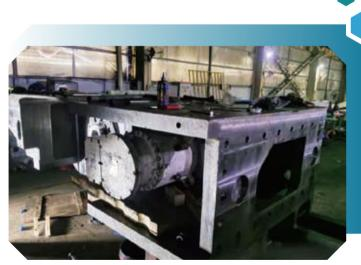
mining machine. The axial flux motor, a power component of the coal mining machine in this project, is made of high-strength steel materials which require strict quality control in welding while precise pre-heating is indispensable in the processing of thick plates to avoid cracks. Apart from such specifications, the customer has very stringent requirements on machining accuracy.
