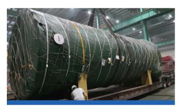
The project was designed by Air Liquide, while Jingjiang Daming Heavy Industry has provided the "one-stop" processing services of high standard cutting, grooving, rolling, welding and seamless inspection. All processes were finished strictly in accordance with customer standards and were finally examined and accepted.
